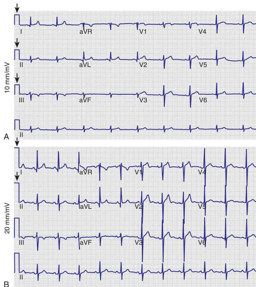
Figure 14-4 A, Normal 10-mm/mV calibration. Note the box-shaped mark to the left of the complexes (arrows); this is a graphic representation of the calibration for the tracing. This parameter should be routinely noted before electrocardiographic interpretation. Note the change in B. B, Abnormal 20-mm/mV calibration. The calibration in this tracing was (inexplicably and unexpectedly) changed to 20 mm/mV by the ECG, not by the operator. When compared with a baseline ECG, it appeared that the patient had developed voltage criteria for left ventricular hypertrophy as well as ST segment elevation. A was recorded minutes later with correction of calibration to the standard 10 mm/mV and was unchanged from baseline tracings.
