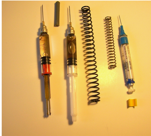
Figure 4. Retrieved material from auto-injectors. From left to right: pre-2010 EpiPen carpule, pre-2010 rubber needle cover, post-2010 EpiPen carpule, auto-injector springs (2 types), Twinject syringe with yellow clip. Photograph courtesy C. Weil.
