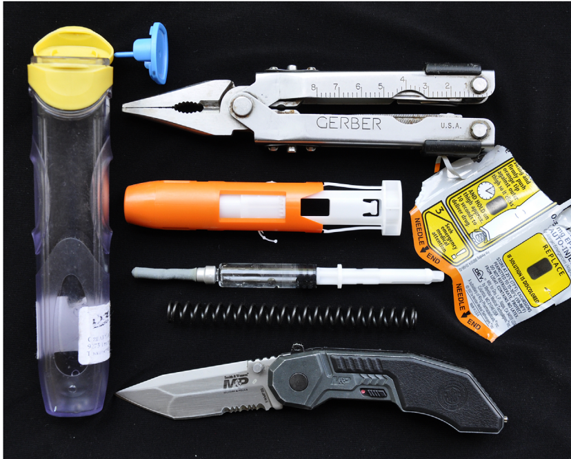
Figure 9. Tools used to remove the carpule, the carpule itself after removal, and the opened auto-injector shell of a post-2010 EpiPen. Photograph courtesy F. Baty.
