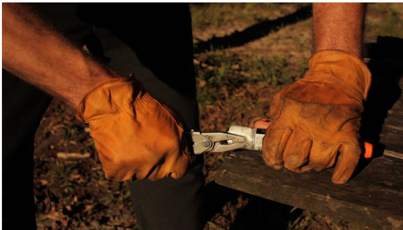
Figure 8. Pry back sheath less than 50%. Photo credits: Caleb S. Varnadoe, David Fitzpatrick.
