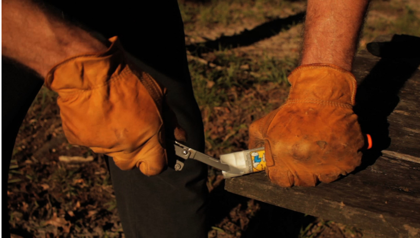
Figure 5. Insert knife edge between rear and sheath of unit. Photo credits: Caleb S. Varnadoe, David Fitzpatrick.
